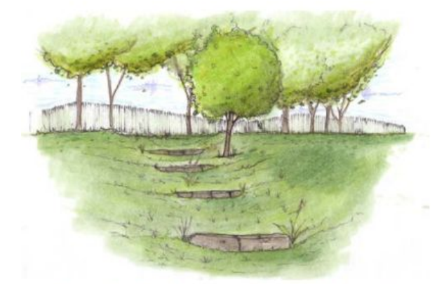
Figure 2. Check dams within a swale slow the flow, allowing sediments to settle out and some infiltration to occur.
