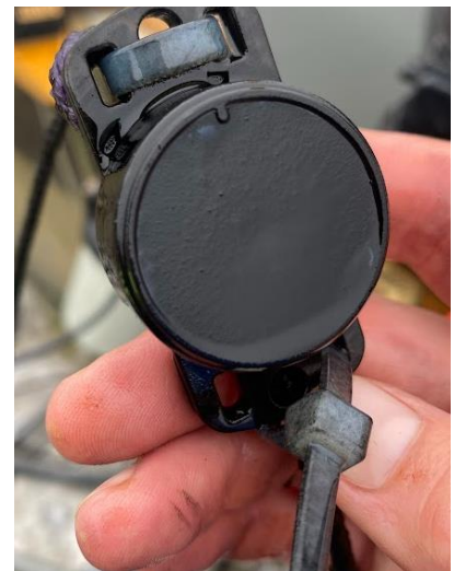
Photo 1. Sept 26 th : 10m temperature sensor iron-sulfide coating
