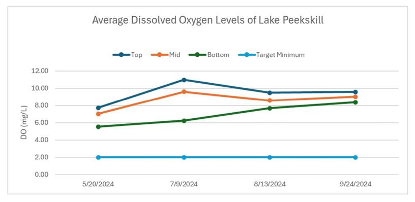
With the aeration system, the average dissolved oxygen levels remained high throughout the sampling period. However, in Sampling Point 2, the dissolved oxygen level did dip slightly below 4 mg/L at the bottom in May but increased and remained between 5.13 mg/L - 7.9 mg/L for the remainder of our in-situ sampling dates.
