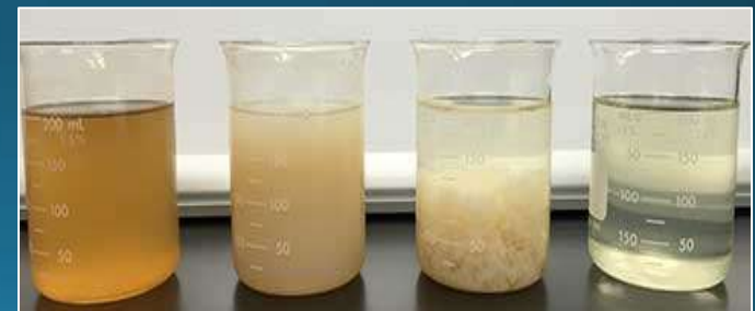
Photo demonstrates flocculation and water clarity process ( http://www.devrkenterprises.com/coagulant-chemicals.htm )
